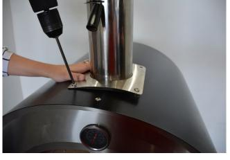
3. Put the chimney in place and drill the screws to secure the chimney to the pizza oven.
