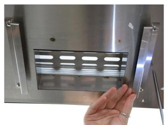
4. Under the pizza oven next to the ash exit, secure the two small rails. Slide in the ash tray.
